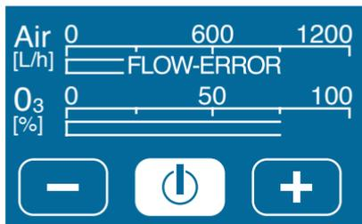
If airflow through the ozonizer drops below 75 litres per hour, ozone production will shut down to prevent overheating. Please provide sufficient airflow to the ozonizer, removing any blockages.
