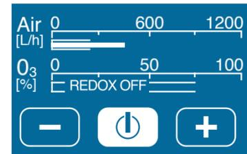
When using a redox controller, ozone production is turned off automatically once the target redox potential set on the redox controller has been reached. When the redox potential drops below the set value, ozone production is resumed.
