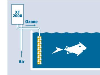
There are two fastening clips on the reverse side of the ozonizer. These may be used for wall mount. It is recommended that the ozonizer be mounted above the water level. This will prevent water from flowing back into the ozonizer, eg. in the event of a power failure.
