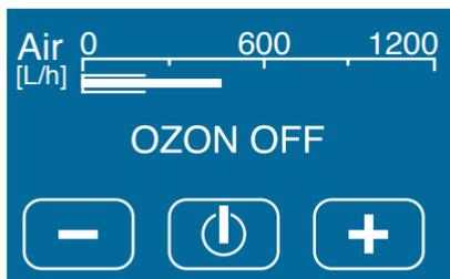
The upper bar graph («Air») indicates the amount of airflow through the ozonizer in litres per hour.
