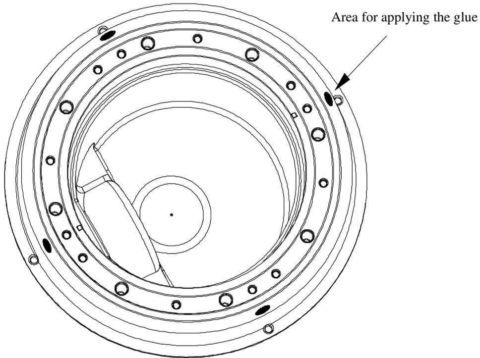
In order to secure the position of the gasket during applying the foil, the seal should be fixed to the body on approx. 4 glue areas (see drawing).
